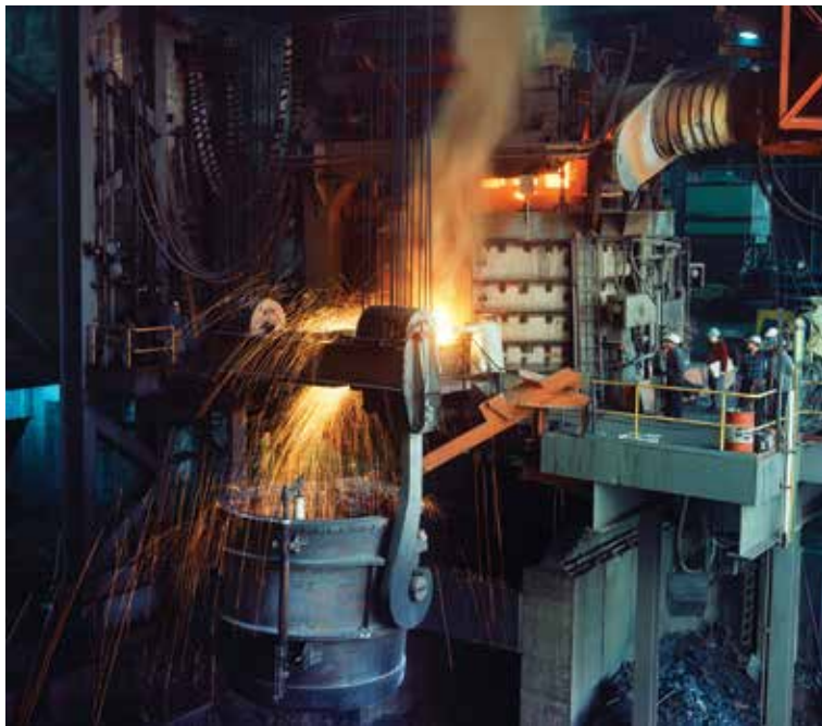
"C" Furnace Tap
